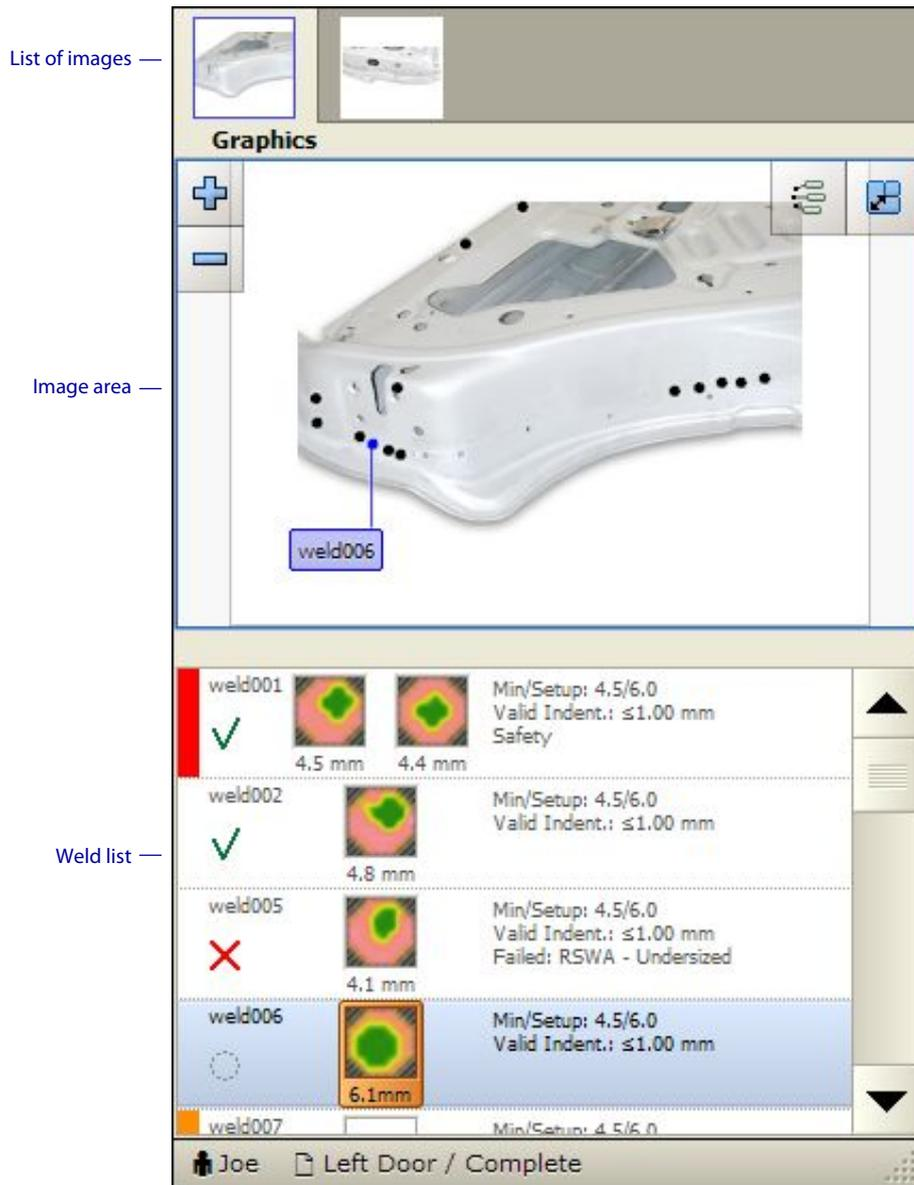
Figure 3.11 Array Explorer in Part Inspection mode
