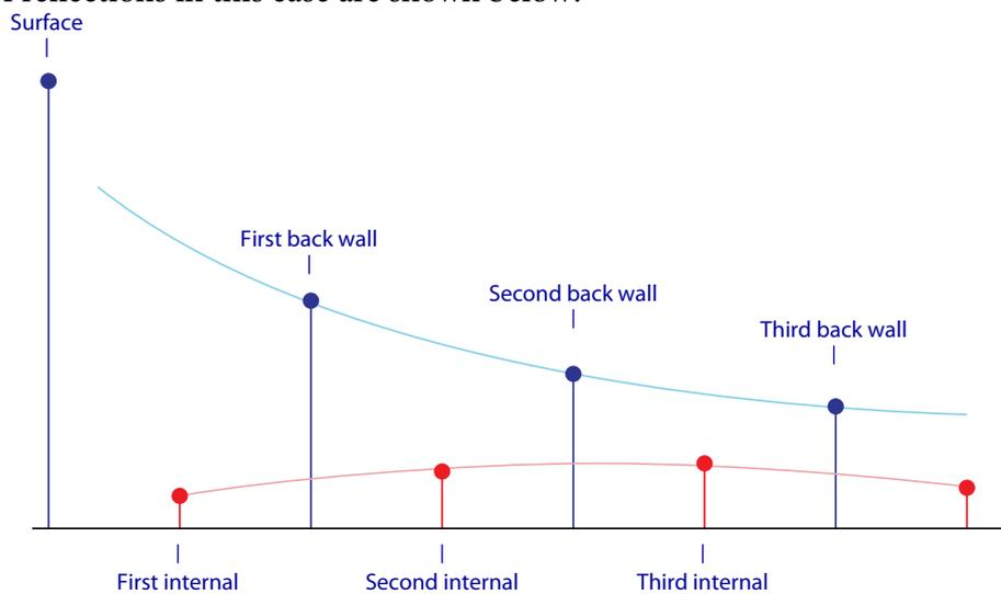
Then the Secondary Echo mode is activated, the presence of the secondary echoes is detected. There are three levels of the sensitivity: Subtle, Moderate, and Full. In the full mode, the sensitivity of the algorithm is very strong, so that even small reflections are detected. In the subtle mode the algorithm is least sensitive, the secondary echo signal
