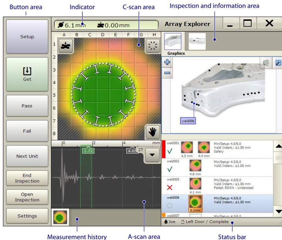
Figure 3.1 Main Array Explorer Window
