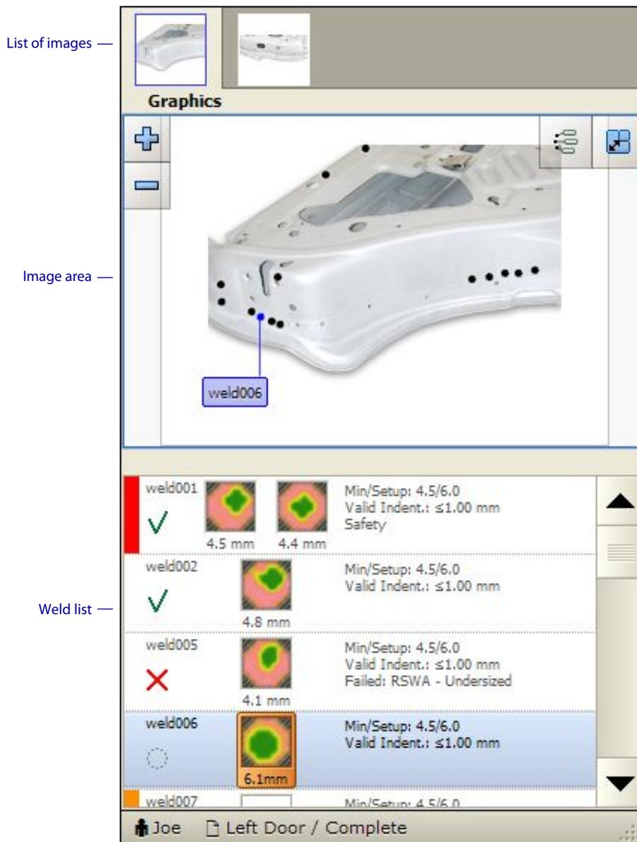
Figure 3.11 Array Explorer in Part Inspection mode
